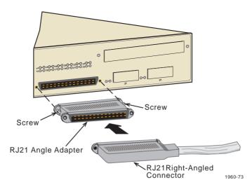
Figure 3-9 Connection Using the RJ21 Angle Adapter
